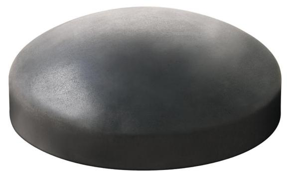
Die formed heads made in Ohio will have a dish radius equal to 80% of the diameter and an inside corner (knuckle) radius of 3T (T = thickness) or 7% of the diameter, whichever is greater.
